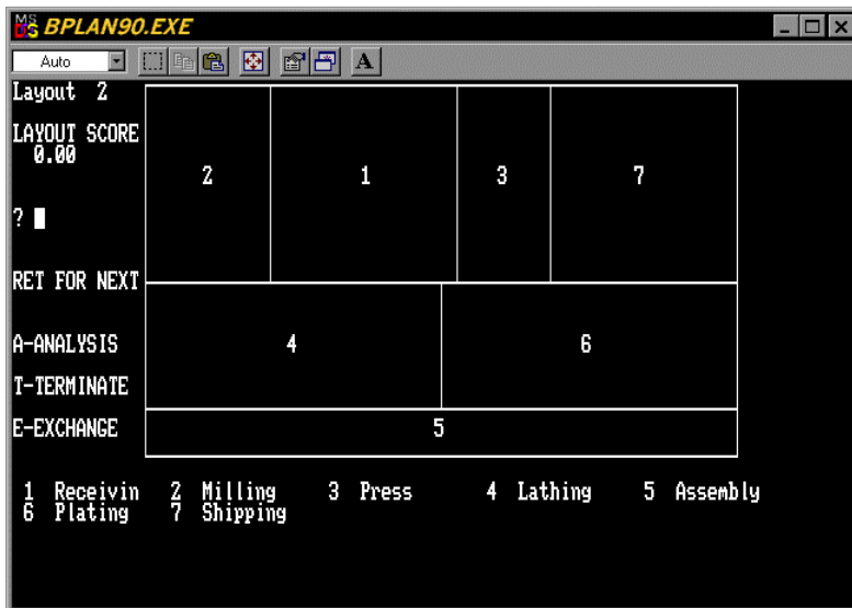
Figure 15.39. BLOCPLAN Layout for the Tompkins Example with Numerical Data
